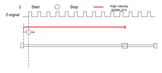
**Mode -1:** Search for homing point in **positive direction** at **high velocity**. Move in **negative direction** after torque reaches the value set in Pr5.39, stops when torque is
