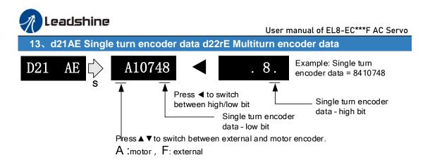
For 23-bit encoder, single turn encoder data =  $0 \sim 8388607$ .Each value corresponds to certain position in a single revolution of the rotor, clockwise motion as negative, counter clockwise motion as positive. When counter clockwise single turn data > 8388607, multiturn data +1, clockwise single turn data < 0, multiturn data -1.
