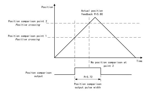
Diagram below shows travel time between 2 points is smaller than output pulse width
