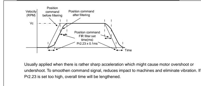
\*\*Please wait for command to stop and after filter idle time to modify Pr2.23. Filter switching time = (Pr2.23 set value x 0.1ms + 0.25ms)
