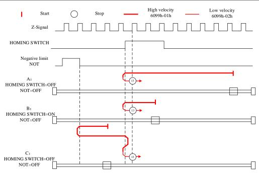
Diagram A: Homing switch & negative limit switch = OFF
