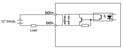
Power supply is provided by user. Please be aware that reversed power supply polarity might cause damage to the driver.
