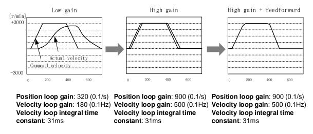
Servo driver gain adjustment is done in combination with a few other parameters (Inertia ratio, Position loop gain, Velocity loop gain and Filters settings). These parameters will have an effect on each other so it always advisable to tune each parameter accordingly in order to achieve optimal machine performance. Please refer to the steps below
