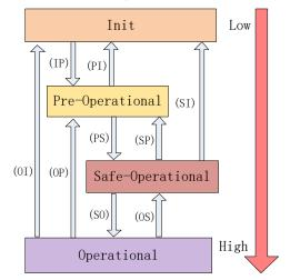
Figure 7.3 EtherCAT state machine transitions
