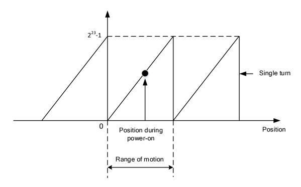
If power is turned off at position as shown below and power on when motor reaches the position below. Motor range of motion changes as shown below.
