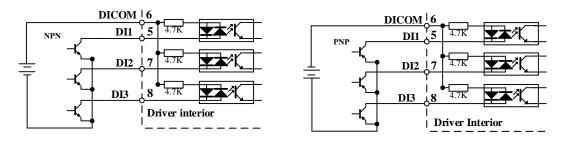
Please prepare switching power supply with output of 12-24VDC, current≥ 100mA;
