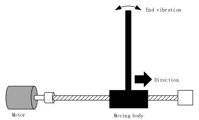
If the mechanical has an end that is long and heavy, it might cause end vibration at emergency stop and affect the positioning. Usually happens on long armed axis with loose end. The frequency is usually within 100Hz which is lower than mechanical resonant frequencies. It is called low-frequency resonance which can be prevented by applying low frequency suppression function.
