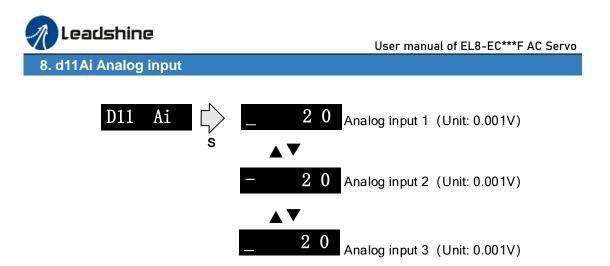
3 analog inputs can be monitored through d11. Left most bar at the top: 1<sup>st</sup> analog input; at the middle: 2<sup>nd</sup> analog input; at the bottom 3<sup>rd</sup> analog input. Points on 4<sup>th</sup> and 5<sup>th</sup> value means negative value.
