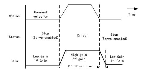
1<sup>st</sup> gain (Pr1.00-Pr1.04) and 2<sup>nd</sup> gain (Pr1.05-Pr1.09) switching can be realized through manual and positioning mode. Switching condition is set through Pr1.15. Gain switching is invalid under standard mode.
