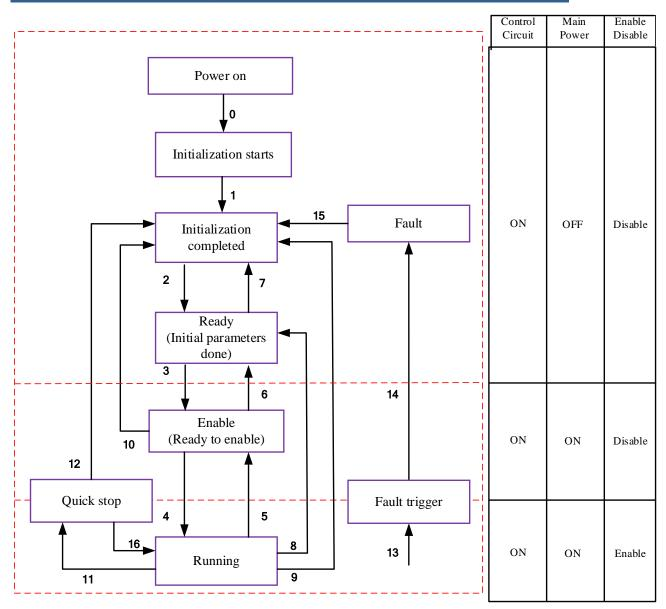
Figure 5.1 EL8-EC 402 State Machine switchover diagram
