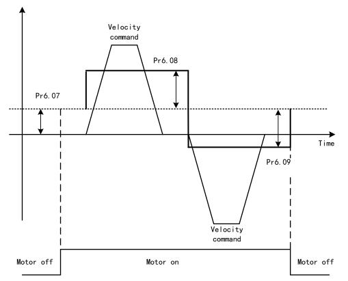
Vertically loaded axis: A constant eccentric load torque is applied on the motor. By adjusting Pr6.07, positioning deviation due to different motional direction can be reduced. Belt-driven axis: Due to large radial load with dynamic frictional torque. Positioning time delay and deviation can be reduced by adjusting Pr6.08 and Pr6.09.
