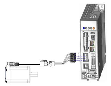
Example of motor power cable connection using an AMP electrical connector *Please connect the wires to corresponding terminals as labeled.*
