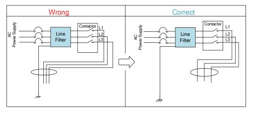
Ground wires inside an electrical cabinet
