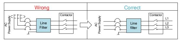
Separate the ground wire from the line filter and the main power supply cable.
