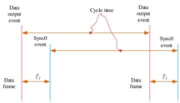
Figure 7.2 High performance synchronization mode
