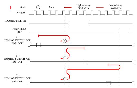
Diagram A: Homing switch & positive limit switch = OFF
