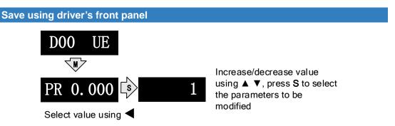
After modifying the selected parameter to desired values, press **S** to confirm and save the changes. If the parameter is modified but user does not want to save the changes, press **M** to exit without saving. Some parameter modifications will only take effect after the driver is restarted.
