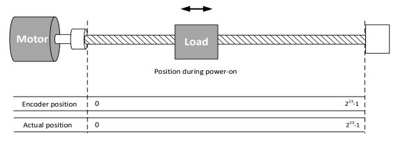
When electronic gear ratio = 1:1, 607Ch = 10000:
