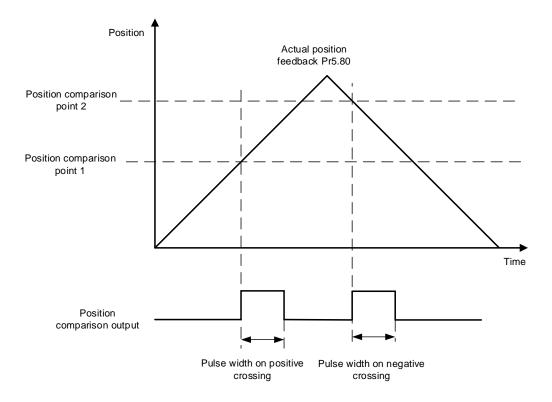
When multiple position comparison points are set, make sure the travel time between 2 comparison points are larger than the output pulse width as position comparison will be temporarily disabled during output.
