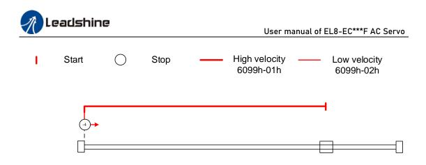
**Mode -3:** Search for homing point in **positive direction** at **high velocity**. Move in **negative direction** after torque reaches the value set in Pr5.39, stops when torque is gone. Homing done signal delivers after the time value set in Pr5.37
