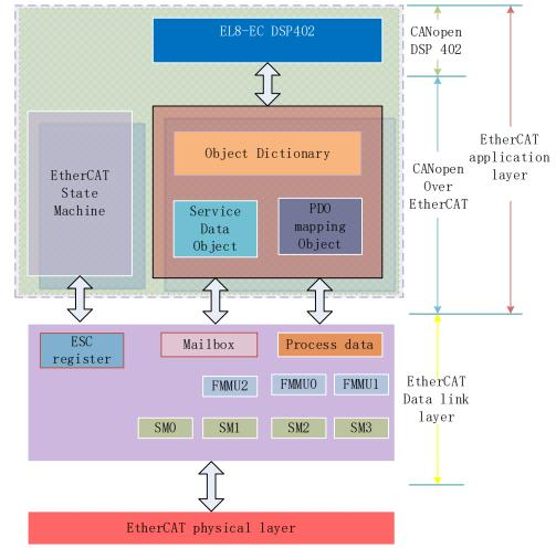
Figure 7.4 Structure of EL8-EC network module
