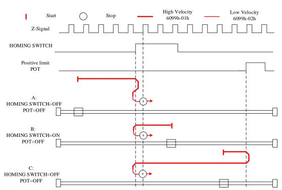
Diagram A: Homing switch & positive limit switch = OFF
