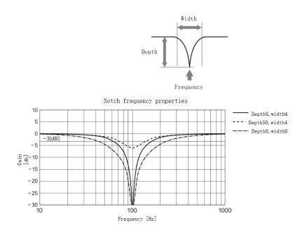
If the \_\_\_\_\_ from mechanical properties analysis tool doesn't show any obvious peak but vibration did occur, it might not be due to mechanical resonance, it may be that servo gain has reached its limit. This kind of vibration can't be suppressed by using notch filter, only by reducing gain and torque command filter time.
