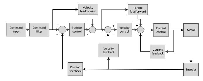
Inner control loop demands higher responsiveness. In order to avoid system instability, please tune in accordance to this principle. Current loop gain usually satisfies the responsiveness demand without tuning. When gain adjustment is done under position control mode, in order to keep the system stabile, position and velocity loop gain have to be increased at the same time to make sure the responsiveness of the position loop is lower than velocity loop.
