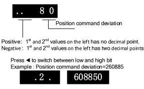
High bit:  $1^{st}$  and  $2^{nd}$  values on the right has two decimal points Low bit:  $1^{st}$  and  $2^{nd}$  values on the right has no decimal point.
